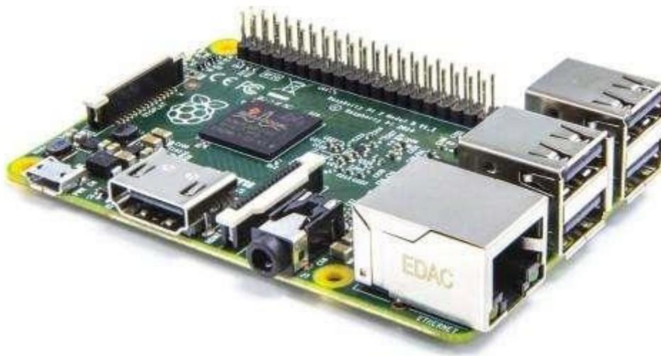
Figure 5 Single-board computer Raspberry PI [25]
